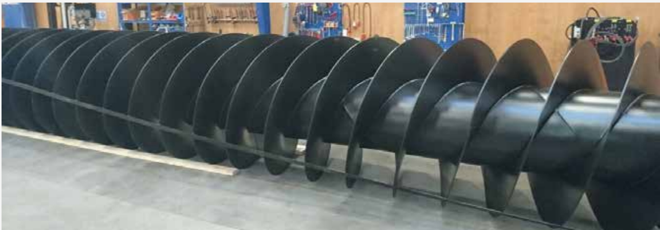
Case: 26161 from www.bema.as (Archimedean screw)
